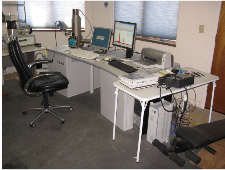
Figure 5-11. Scanning Electron Microscope (SEM) with Energy-Dispersive X-Ray (EDX) Spectroscopy Capability. The SEM is the tall vertical cylinder. The EDX is the instrument just to the left of the SEM.
