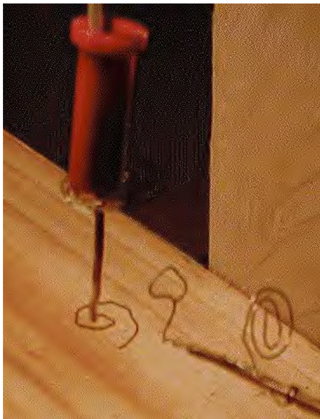
Figure 4 The rigid cathode-anode setups for two cells. The setup from the cell #1 is on the left (vertical) while the setup from the cell #2 is on the right (horizontal). Spiral anodes can also be seen.
