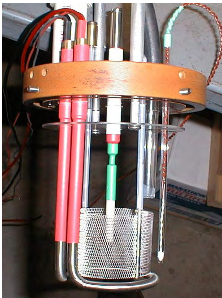
Figure 3 Electrodes and other components mounted on the lid. The ring below the anode is the ohmic heater, the vertical glass tube on the right contains the thermistor. The transparent antislashing baffle can be seen below the lid. The side screws were used to mount the lid rigidly on our polycarbonate cell (note the deep groove on the lower surface of the lid). The tip of the tungsten cathode is shown in Figure 4 below. =====
