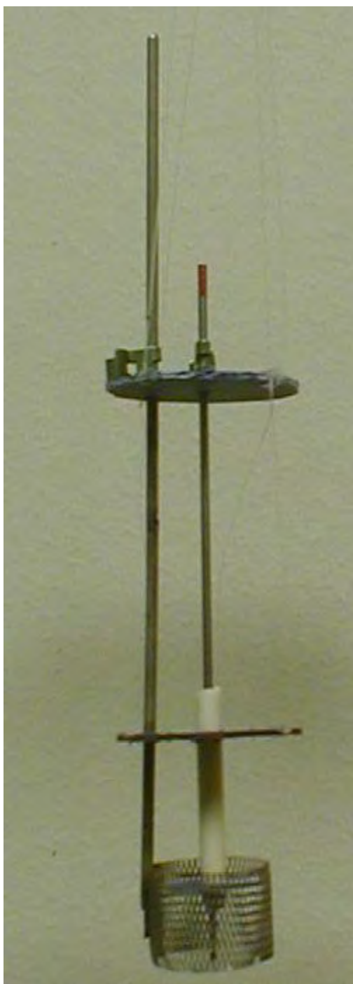
Figure 1 The cathode (shorter tungsten rod) and the anode (welded to the longer Ti rod), suspended by a nylon thread, are being lowered into the beaker. Rigidity was assured by two plastic disks (sterilite remains rigid at 100 C). The second function of the lower disk was to act as an antispashing baffle, inside the electrolyte.
