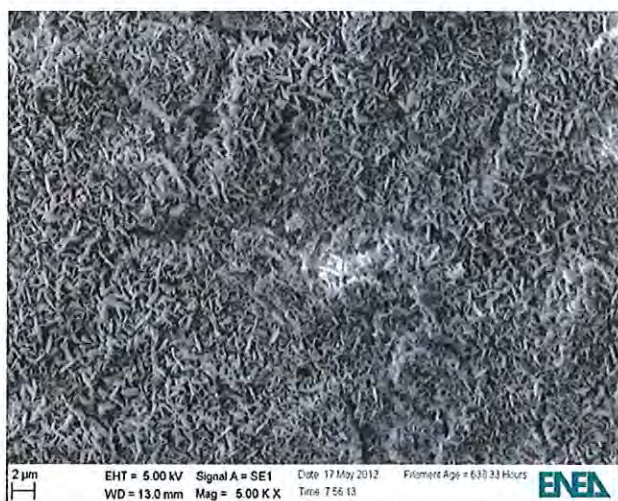
Fig. 14a. SEM image of the electrode surface as it was during the production of excess power.
