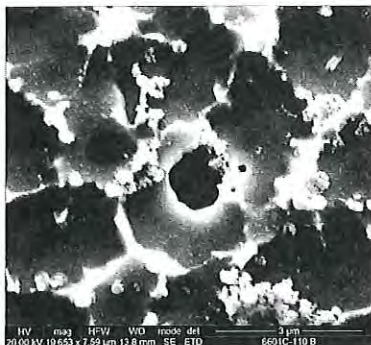
Cathode 1012 negative crystals (AHE)
