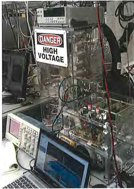
Figure 13. SKINR fabricated high voltage pulsed current power supply. It delivers a 3000 Ampere, 40 microsecond rise time, 100 microsecond width pulse at 1/3 Hz. This produces a 1 Tesla magnetic field pulse on the cathode that is placed between two electromagnetic coils. The coils were also fabricated by SKINR.
