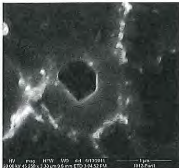
Cathode 1012 negative crystals (AHE)
