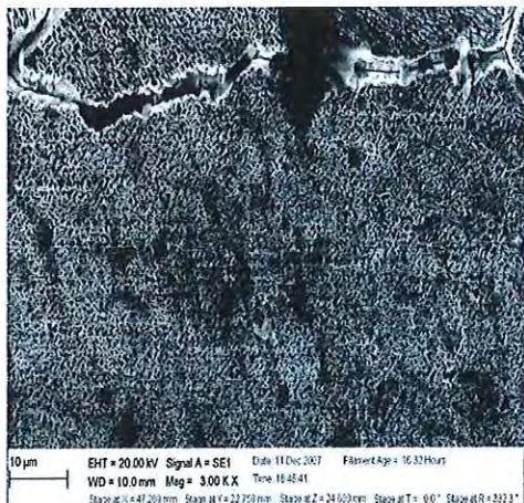
SEM of the surface of #64 electrode giving up to 2500 %.
