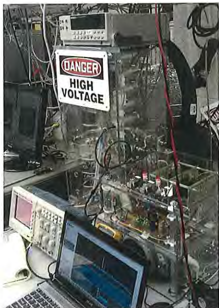
Figure 3. SKINR fabricated high voltage pulsed current power supply. It delivers a 3000 Ampere, 40 microsecond rise time, 100 microsecond width pulse at 1/3 Hz. This produces a 2 Tesla magnetic field pulse on the cathode that is placed between two electromagnetic coils. The coils were also fabricated by SKINR.
